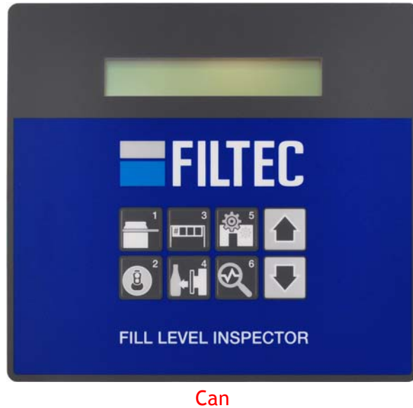
Figure 4-1. Operator Control Panel on the Filtec 3-G
